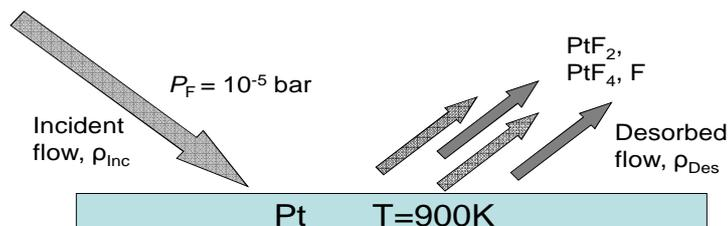
Fig. 1. Gasification of Pt by a flow of atomic fluorine
